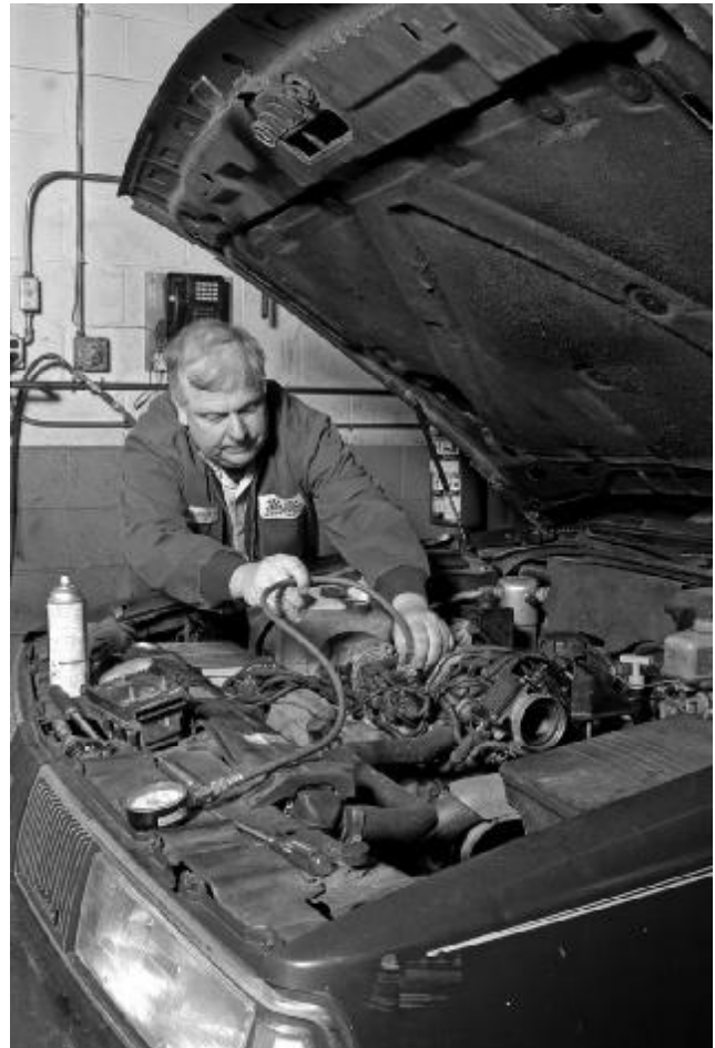
Automotive service technicians use several types of diagnostic tools, including pressure gauges and electronic meters.
